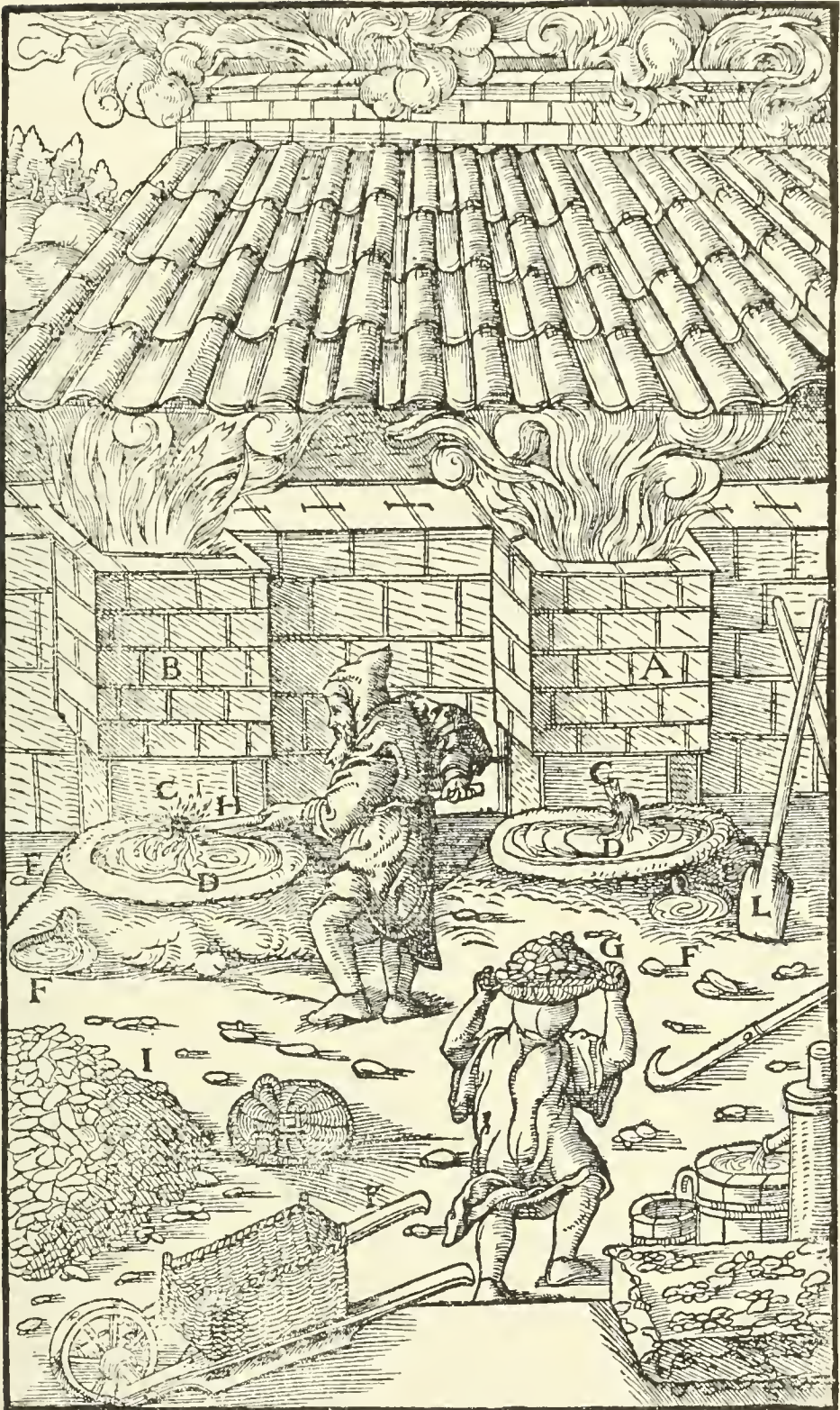
A, B—Two furnaces. C—Tap-holes of furnaces. D—Forehearth. E—Their tap-holes. F—Dipping-pots. G—At the one furnace stands the smelter carrying a wicker basket full of charcoal. At the other furnace stands a smelter who with the third hooked bar breaks away the material which has frozen the tap-hole of the furnace. H—Hooked bar. I—Heap of charcoal. K—Barrow on which is a box made of wicker work in which the coals are measured. L—Iron spade.
